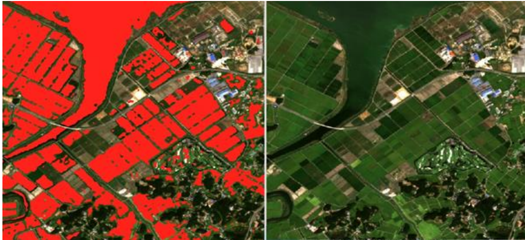
Figure 6. VH backscatter 2018 water mask via thresholding
