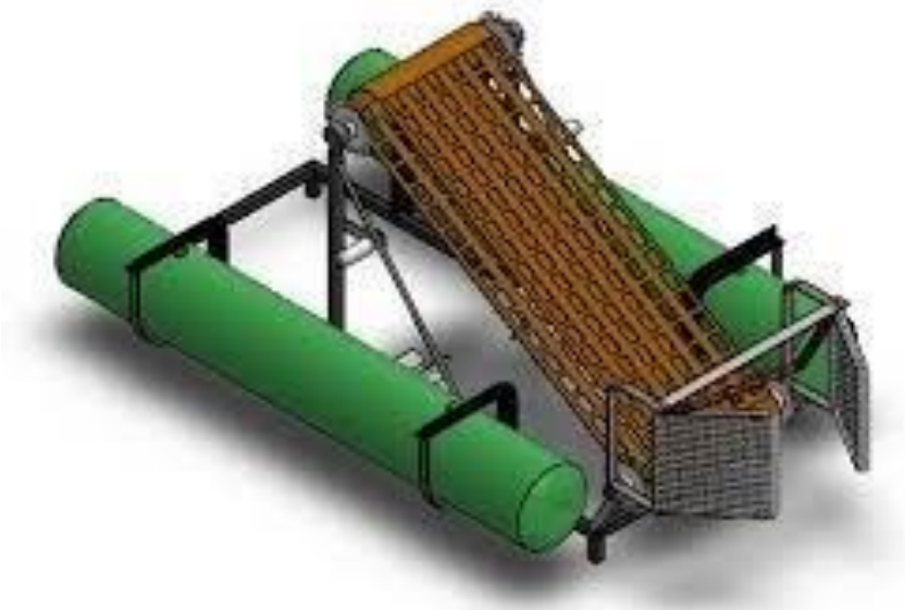
Fig. 2: 3D Model of Water Body Cleaning Machine.
