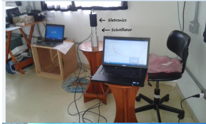
Fig. 1: View of gamma scintillator with associated electronics and computer
