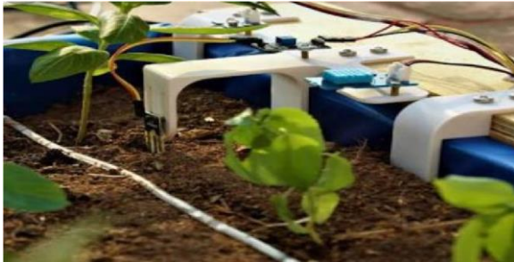
Fig. 5: DHT11 Sensor in Agricultural Field.
